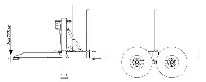
The vertical load on the towing eyelet may not exceed the load for which the towing vehicle's towing device is approved, or a maximum of 2,000 kg. The load on the towing eyelet is governed primarily by four factors:
