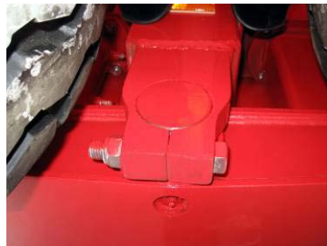
Bolts on either side of the bogie
